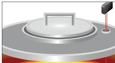
Level detection of melted aluminum liquid.
